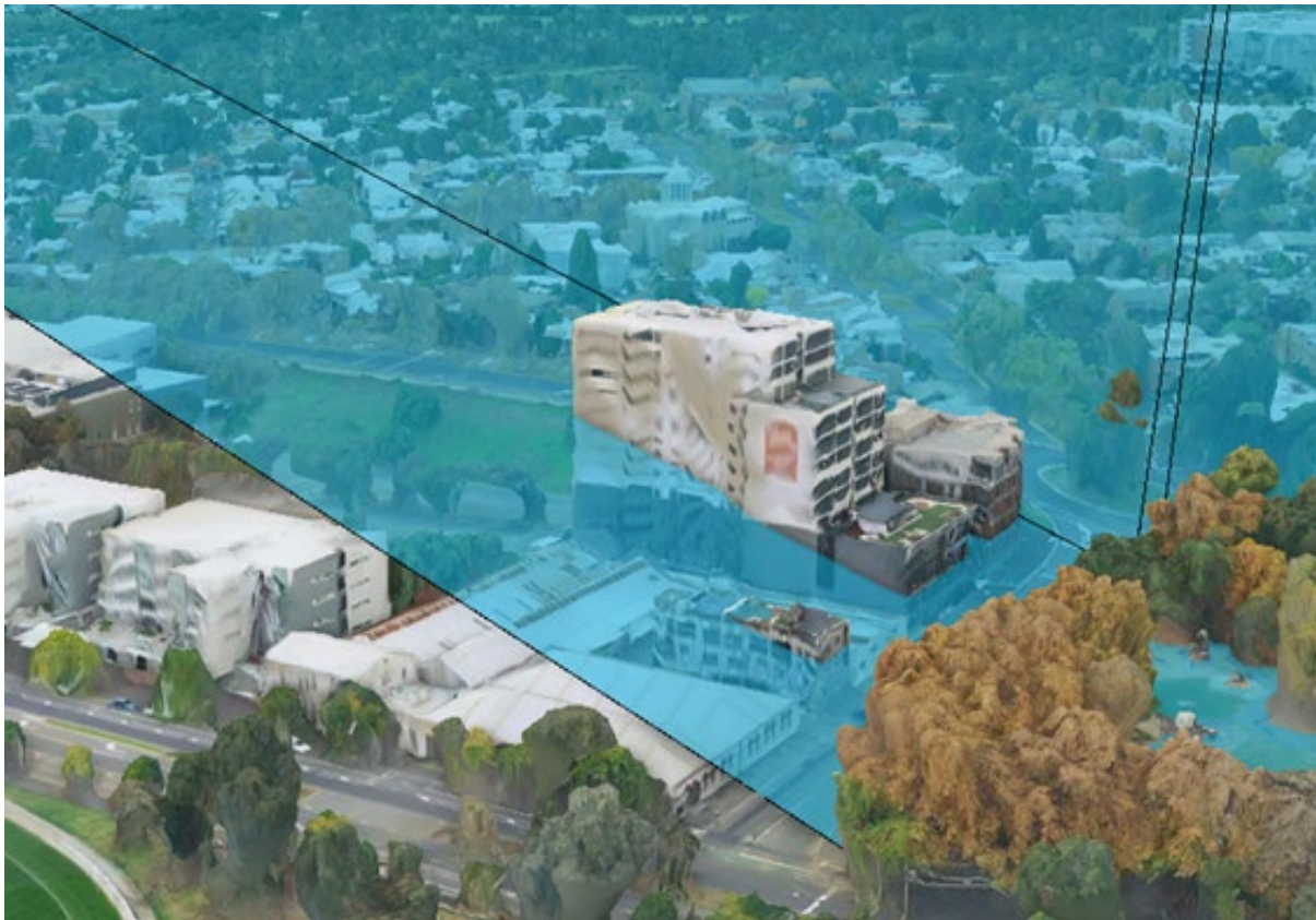
Figure 5.4 – Detail of the solar surface for Gardiner Reserve (Note the buildings penetrating above the surface: these buildings therefore have the potential to overshadow the park)
