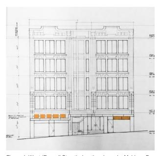
Figure 4. West (Russell Street) elevation drawn by Meldrum Burrows & Partners in 1972. Coloured in orange shows openings to be bricked. (PROV Public Building Plan VPRS8044/P/3)
